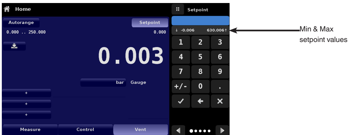
Figure 6.4.1.2.1 Numeric Keypad Setpoint Entry
